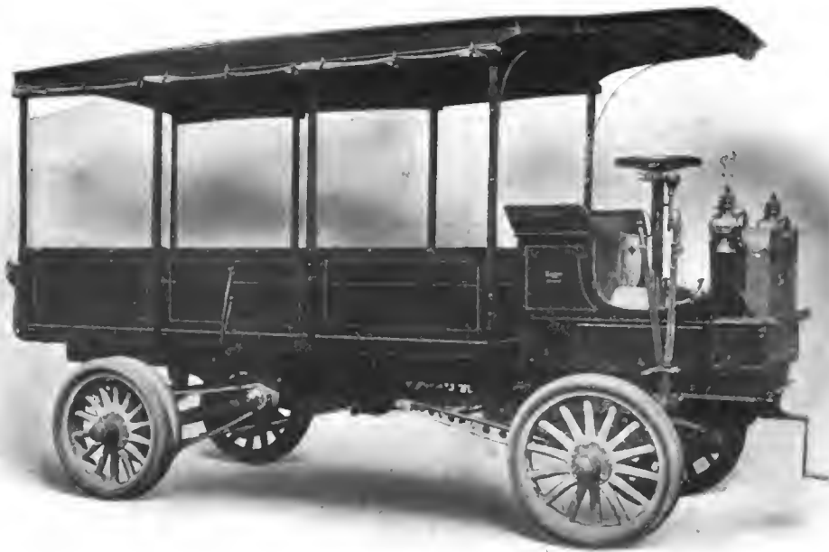
LOGAN THREE-TON TRUCK, MODEL S, WITH OPEN BODY, 4 CYLINDERS, 40-H.P. Logan Construction Co., Chillicothe, O.
